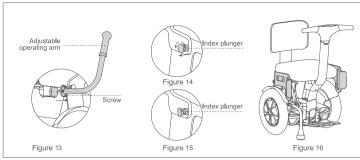
♠ Loosen the set setscrew (see Figure 13) to remove the adjustable operating arm from the body. Pull outward and rotate the index plunger (see Figure 14) and get the mount stuck and loosen the index plunger (see Figure 15); rotate the armrests to horizontal position (see Figure 16-arrow). Pull outward and rotate the index plunger and release it when a click sound is heard. Then the armrest is folded .
