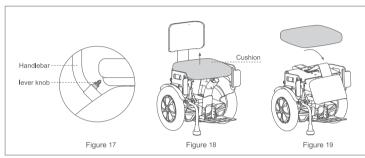
Rotate the lever knob. After hearing a "click", pull out the handlebar (see Figure 18), tear up the cushion tape (see Figure 18), remove the cushion. Then rotate the backrest in the direction follow the arrow in Figure 19. fold the backrest, and then attach the cushion to the body to complete the folding.
