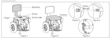
1 Take A6TS from the packing container. Align the screws on backrest hinge to the screw holes and body holes, tighten screws (see Figure 1) and stick saddle to frame(see Figure 2). Pull outward and rotate the index plunger (see Figure 3) and get the mount stuck and loosen the index plunger (see Figure 4); rotate the armrests to horizontal position(see Figure 5 - arrow). Pull outward and rotate the index plunger and release it when a click sound is heard.
